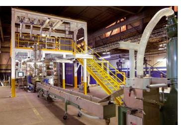
exceed 20%, causing substantial reductions in extruder throughput. The new PLC control automatically adjusts the timing of the reciprocating ram which stuffs material into the screw. Changes are made in accordance with variations in extrusion drive amperage caused by changes in material bulk density. Since the ram cycle governs the rate at which material is fed into the extruder, the controller ensures that production will continue at the maximum level without the need for operator intervention.
