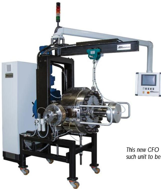
*This new CFO continuous melt filter from ADG Solutions is the first such unit to be made in the U.S.A.*
