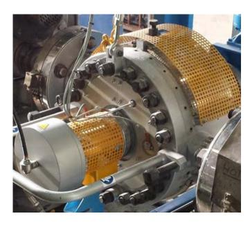
New control programming on continuous, self-cleaning screen changers from ADG Solutions dramatically reduces polymer required to purge filtered contaminants.
