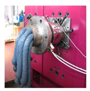
Shredded material is fed into the feed throat of the densifier. Twin counter-rotating screws compact the material, raising its temperature to between 380 and 390°F and forcing it out the die.
