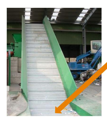
FLAT PART UNDER THE FLOOR TO BE FED WITH FORK TRUCKS OR FRONT END LOADER
