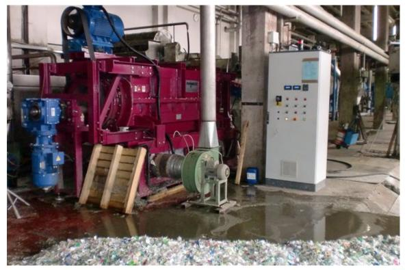
LAST WASHING OF THE POLYMERS WITH WATER USING CENTRIFUGE TECHNOLOGY
