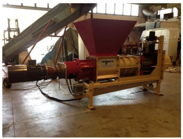
SCREW PRESS TO REDUCE MOISTURE <5-7% TO SQUEEZE OUT THE WATER
